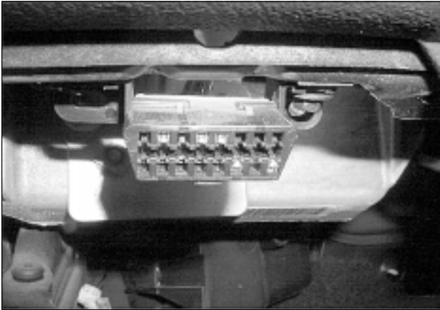
Figure 5 The OBDII port located under the instrument panel can be used to obtain diagnostic data.
