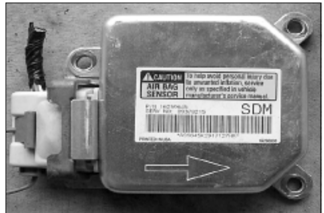
Figure 1 The GM black box or Sensing Diagnostic Module (SDM) is shown here.
