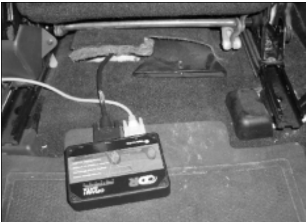
Figure 6 The Crash Data Retrieval (CDR) tool can also be connected directly to the black box commonly located under the driver's seat as shown here. The second cable is connected to a laptop computer.
