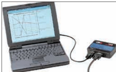
As shown above, the Vetronix CDR System is a peripheral connected to a PC's serial port. The PC is loaded with proprietary Vetronix software.
